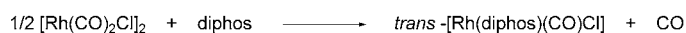
Scheme 4. Synthesis of trans -[Rh(diphos)(CO)Cl] Complexes 7–9 from [Rh(CO) 2 Cl] 2 and the diphos Ligands pbpb , nbpb , and cbpb
